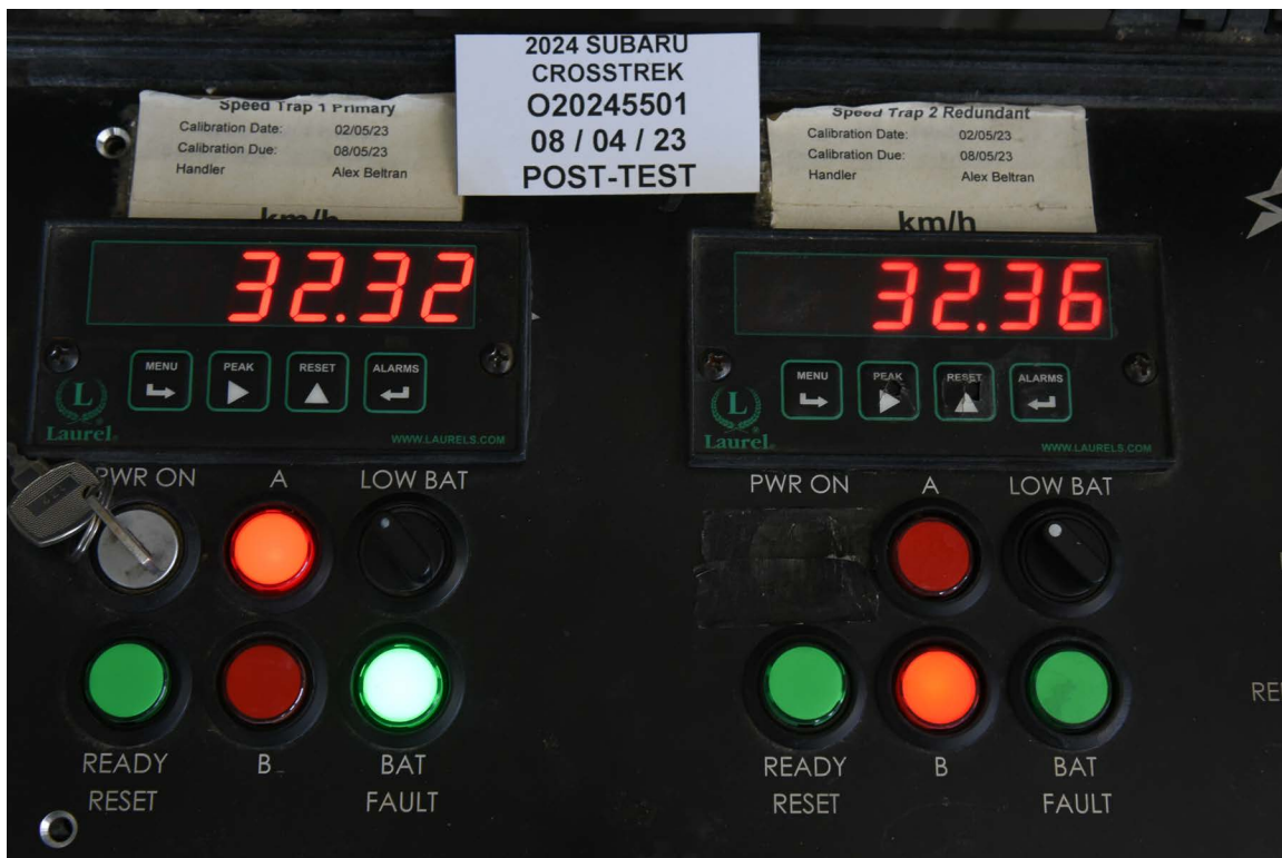
FIGURE 64. Post-Test Primary and Redundant Speed Trap Read-Out
